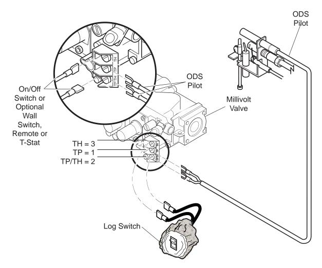
Figure 17 - Wiring Diagram
